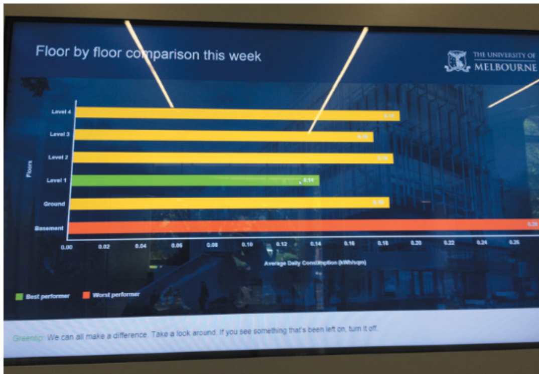
Figure 10.16 Average daily energy consumption depicted on a public display for a building at the University of Melbourne. Green is best performer, yellow is in the middle, and red is the worst performer.
