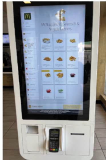
Figure 3.6 A self-ordering kiosk found in many fast-food restaurants that uses a card metaphor as part of the interface. Each food or drink item is displayed on its own card with associated description and price. This enables the customer to easily select items they want to purchase from the category types in the card matrix while also going back and forth between the other high-level categories (e.g., burgers, vegan, cold drinks), shown down the left side of the display.
