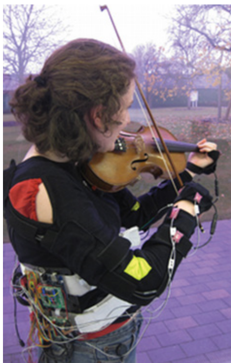
Figure 7.22 The MusicJacket with embedded actuators that nudge the player to move their arm up to be in the correct position
