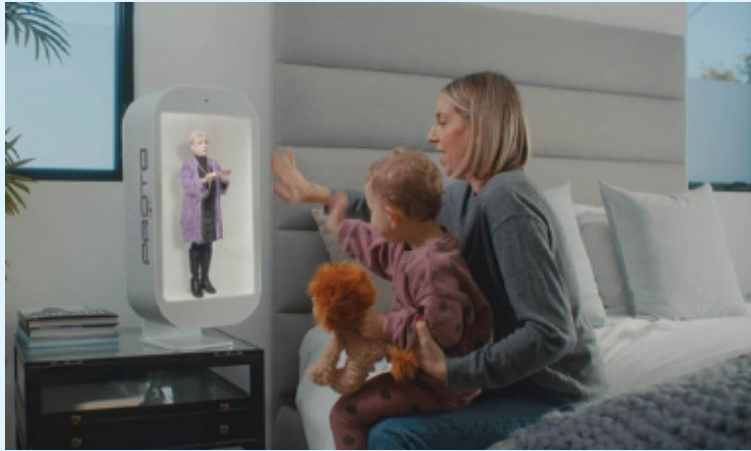
Figure 5.13 Talking with a 3D video of granny in a box (Proto M). The embedded camera at the top of the box faces the mother and child so that Granny can see and hear them in real time. They can also see and hear Granny.
