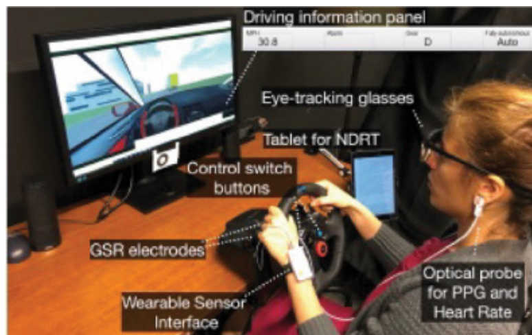
Figure 14.3 User study setup. This custom driving simulator consists of a 30-inch monitor, a Logitech G29 steering wheel, and 10.5-inch Apple iPad Air on which the non-driving tasks are displayed. For switching between the automated and manual control of the vehicle, the participant needs to press the two blue buttons on the steering wheel simultaneously. The participant wore a pair of eye-tracking glasses and a wearable device with sensors for collecting skin.
