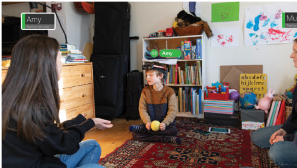
Figure 5.16 PeopleLens: a head-mounted device that enhances a blind child's spatial awareness of those around them
